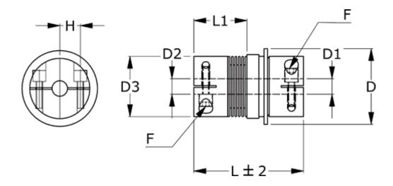
D = 109 Nom. torque NM (Tkn) = 200NM overload torque range 2
